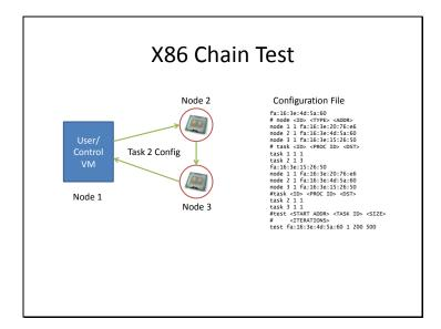
To test the system, a basic test platform was put together chaining two X86 VMs together. The right side of the slide should the configuration file for the test which the controller used to send command frames to each node. Three tasks are defined:
