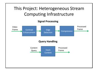
This project investigates a class of computations called stream computing. Stream computing is a general model where computations are defined as a series of sequential operations. Applications that fit well into this model are filtering pipelines such as for signal processing. In addition, basic content queries and responses can be modeled in stream computing.
