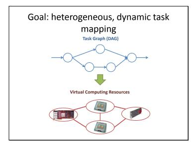
The goal in this project is then to come up with a method of mapping a stream application, typically represented as a directed acyclic graph (DAG), onto a set of heterogeneous computing resources. The solution should facilitate mapping onto heterogeneous nodes as well as be robust to changes in the available computing resources. For instance, if a new FPGA instance is booted, the system should be able to immediately re-allocate work onto it.
