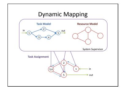
Finally, with the resource model in mind, we would like a method of distributing tasks onto them. The choice here is to use a globally-aware supervisor that examines the task graph of the application as well as the available resources and solves an optimization problem to map the tasks onto the virtual hardware.
