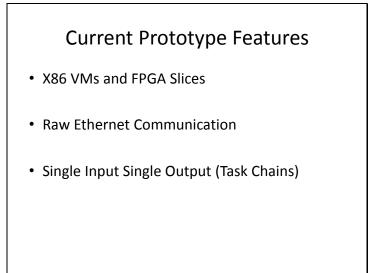
The prototype designed for this course supports a small subset of the desired features. In particular, the focus was on connecting X86 VMs and FPGAs. Thus, only raw Ethernet is supported as a transport and control layer. Further, only single input single output task graphs can be created. In other words, only chains of computations are allowed.
