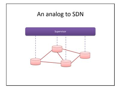
The previous design looks very similar to OpenFlow/SDN. In particular, it consists of a number of computing resources (switches) that forward information based on a globally determined route. The primary differences are:
