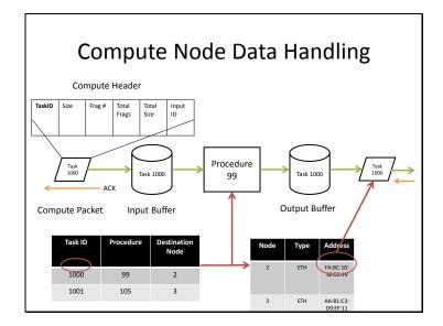
Once the data has been processed, it is passed to an output buffer where the package is broken down into Ethernet frames for the next hop. In this step, a second table is used to translate the destination node to an Ethernet address for transmission.
