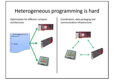
Although heterogeneous resources can be created on SAVI, developing applications on them is a challenge. In particular, two main difficulties are (1) the difficulty of designing high-performance algorithms across different architectures and (2) coordinating work across the resources.
