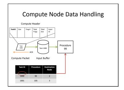
When a compute package is pieced together, its task ID is consulted in a forwarding table that determines the procedure (action) and destination node(s). The hardware performs the procedure defined by the table on the package to produce an output. For now, procedures refer to pre-defined functions in a compute node. Note, a procedure could mean fetch some other data from a table based on the input buffer in the case of content retrieval.
