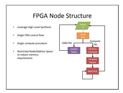
The FPGA hardware was designed using High-level synthesis. This tool converts C code to hardware making development much simpler. A reason to leverage HLS for FPGA nodes is the fact that compute procedures are very easily defined in HLS and a non-hardware designer can create hardware kernels quickly. This is important if many tasks are to be supported on the FPGA hardware.
